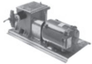
Four headed power Unit. Up to 8 head maximum available. Weight 120 pounds - 4 headed unit. 270 pounds - 6 headed unit
