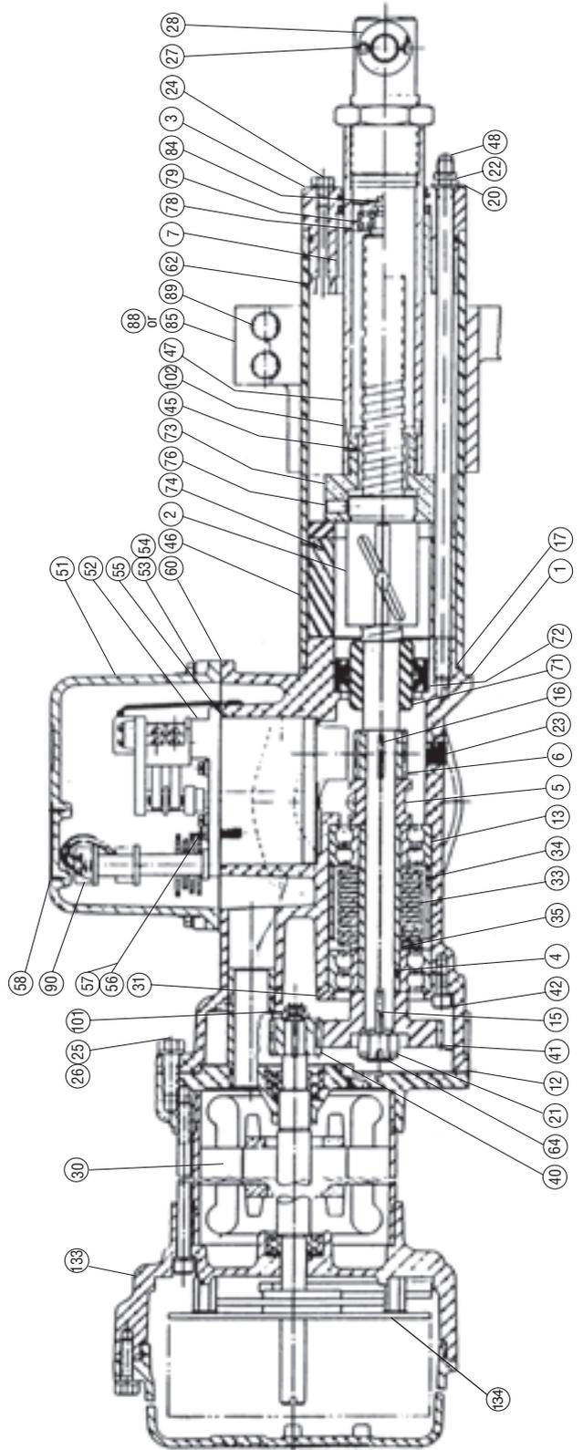
Figure 2 - Ball Screw Actuator Drawing
