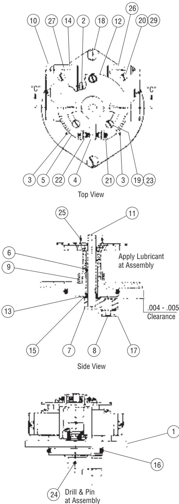
Figure 5 - Thrust Limit Switch Parts Drawing
