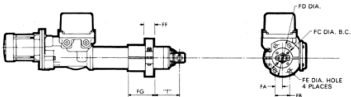
Figure 9 - Face/Flange Mounting
