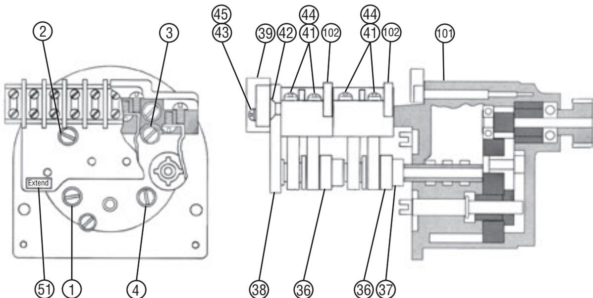
Figure 4 - Geared Position Limit Switch Parts Drawing
